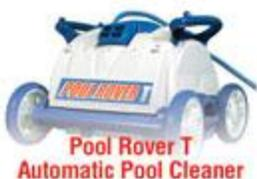
Rather than being powered by suction, pressure-side pool cleaners for above ground pools are driven by water pressure (such as Pool Rover T). These swimming pool cleaners attach to the pressure side return fitting and use the water from the circulation pump to operate. While some pressure-side pool cleaners can operate off existing swimming pool pumps, others require additional pressure provided by a dedicated booster pump.
